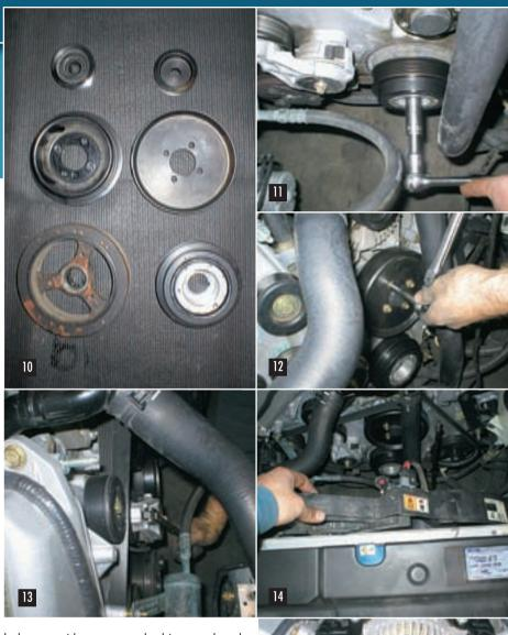
balancer with a new underdrive crank pulley solves those issues. Furthermore, all ASP pulleys are manufactured from billet steel or aluminum, and come standard with a black nitride finish for good looks and durability exceeding factory quality. Knowing that ASP provides a quality product, we chose to install a pulley kit on Joe Pacheco's 2001 Cobra.
