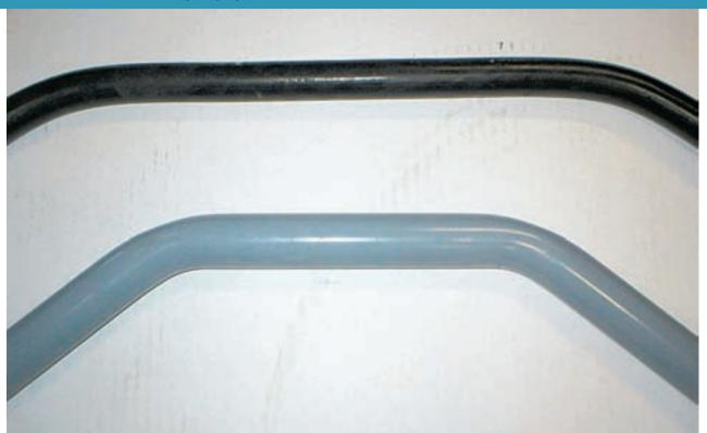
Bigger is often better when it comes to anti-sway bar performance. Here you can see the difference between the stock bar (top) and the larger Progressive bar (bottom). Due to the thicker design of the Progress sway bar, some lowered Mustangs might have slight clearance issues with the steering wheel at full-lock depending on ride height, wheel/tire width, et cetera. Check with GTR for details.
