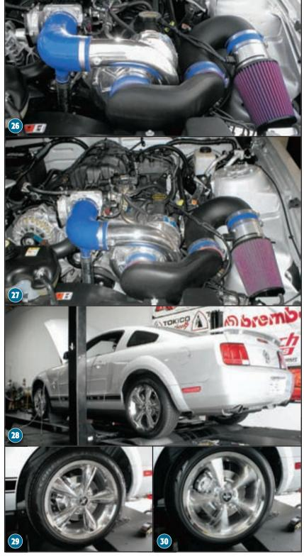
26 Installation is complete. This is what an installed and finished Vortech supercharger kit should look like.
