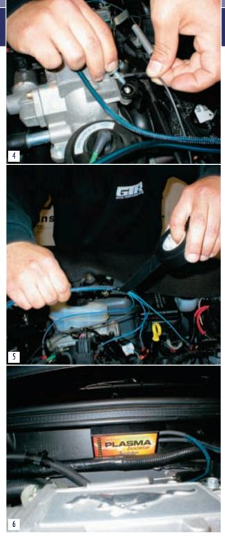
Find a suitable location to ground the Plasma Booster. We sandwiched it under a bolt from the upper intake plenum.
