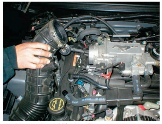
Disconnect the battery and remove the air intake tube leading to the throttlebody for easier access.
