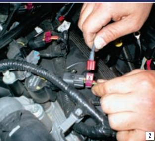
Locate each individual coil and carefully cut the electrical tape to reveal the wires. Use the supplied quick-splice connectors and attach to the left wire of each coil. Use pliers to ensure a proper connection, and repeat this step for all eight cylinders.
