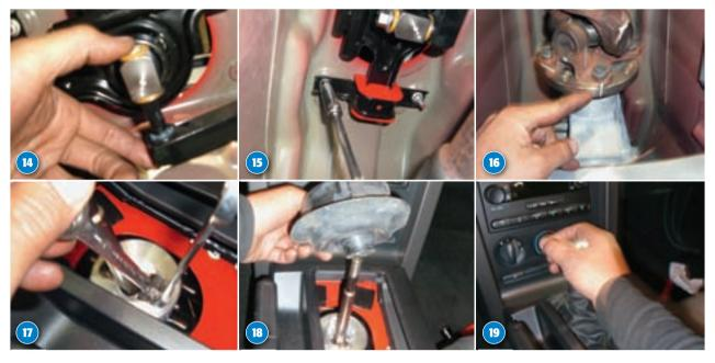
14 Re-connect the shifter lever to the shift rod. Make certain the stock shifter rod bushings are in place.
