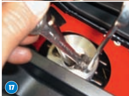
14 Re-connect the shifter lever to the shift rod. Make certain the stock shifter rod bushings are in place.
